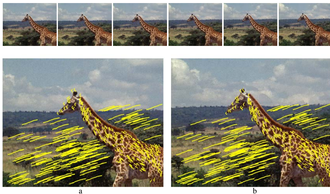
Fig. 18.2. Non-rigid motion sequence. Top row: alternate frames from a sequence in which a giraffe gracefully walks and flexes its neck, whilst the camera pans to match its speed. Bottom row: point tracks showing the motion over (a) the 10 previous, and (b) the 10 forthcoming frames. These tracks are computed using non-rigid factorization and lie in a six dimensional subspace. Note the very different trajectories of the (rigid) background from the (deforming) foreground. Yet these are all spanned by the six basis vectors of the motion matrix. The rank can be accounted for as follows: the sequence motion is effectively that of two planes of points moving independently relative to the camera. The background is a rigid object represented by a plane and contributes 2 to the rank. The giraffe in the foreground is represented as a non-rigid object by a set of l = 2 planar basis shapes and contributes 4 to the rank. Figures courtesy of Andrew Fitzgibbon and Aeron Morgan.
