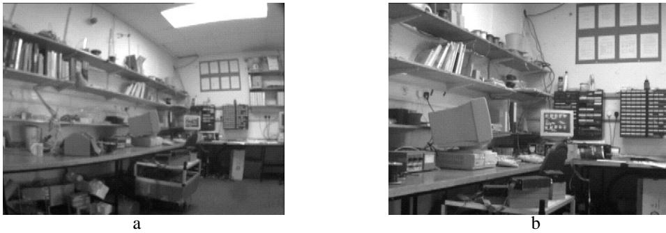
Fig. 7.4. (a) Short vs (b) long focal lengths. Note the curved imaged lines at the periphery in (a) which are images of straight scene lines.
