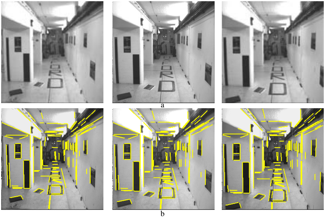
Fig. 16.3. Image triplet matching. The trifocal tensor is computed automatically from interest points using algorithm 16.4, and subsequently used to match line features across views. (a) Three images of a corridor sequence. (b) Automatically matched line segments. The matching algorithm is described in [Schmid-97].
