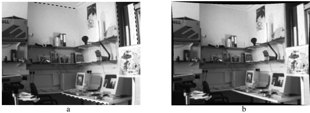
Fig. 7.6. Radial distortion correction. (a) The original image with lines which are straight in the world, but curved in the image. Several of these lines are annotated by dashed curves. (b) The image warped to remove the radial distortion. Note that the lines in the periphery of the image are now straight, but that the boundary of the image is curved.
